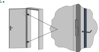
If the gap between the door seal and the door leaf is too wide, you can use a screwdriver or an Allen key to insert the frame-side hinge part deeper into the frame. To do this, first unhinge the door leaf. Adjust the hinge position until the credit card does start to stay put when inserted.
