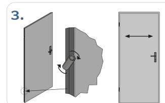
If the door leaf is positioned at a slight angle in the frame, it can be adjusted by turning the hinge(s) accordingly.
